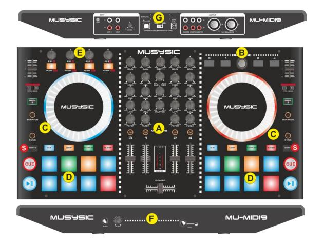
S. SHIFT. Press and hold this button to access secondary functions of other controls on the MD1311
