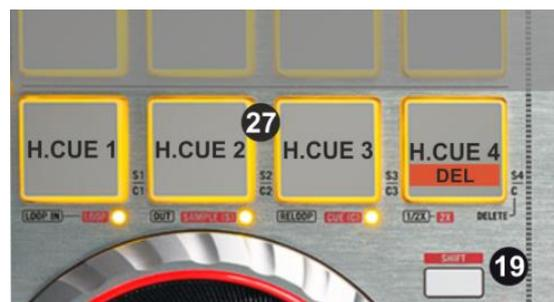
Hold **SHIFT** (18) down and then press the 4<sup>th</sup> PAD from left to enter the **Delete** HotCue mode. The Leds of the 4 Pads will blink (if a HotCue is assigned). Press the Pads to delete its assigned HotCue. Hold SHIFT and then press the 4<sup>th</sup> PAD to return to the HotCues mode.
