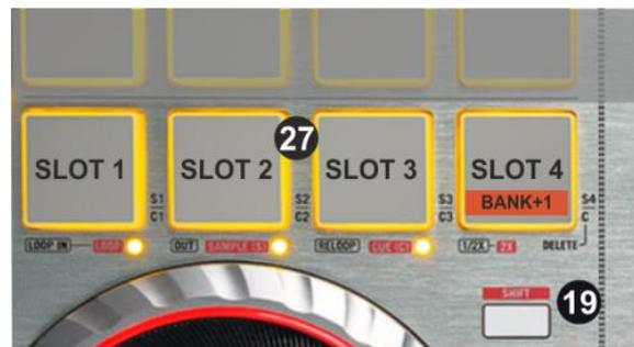
The Leds of the 4 PADs will be lit if a Sampler slot is loaded and will blink if the slot is playing.
