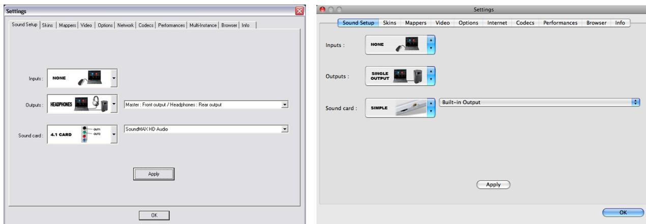
**Inputs** – If using timecode vinyl or CDs to control VirtualDJ, select the appropriate input configuration from this pull-down list. Choices are "NONE", "Single Timecode" for Single control, and "Timecodes" for Dual Control. Setting up VirtualDJ for Timecode use is covered in detail in the "Timecode" section of this guide.
