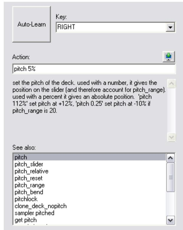
Now you can manually modify the action by adding additional parameters and actions. If you don't want to modify the selected action and want to assign more of your controller's keys to finish the mapping, just repeat steps 2 thru 6 above until you have completely mapped your controller.
