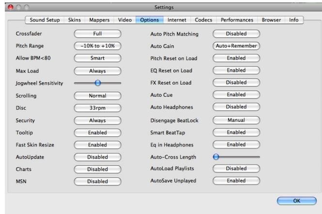
**Crossfader** – This option allows you to select the cross fader curve. There are four different options including: Full, Cut, Scratch, and Smooth. (other curves can be set through plug-ins).
