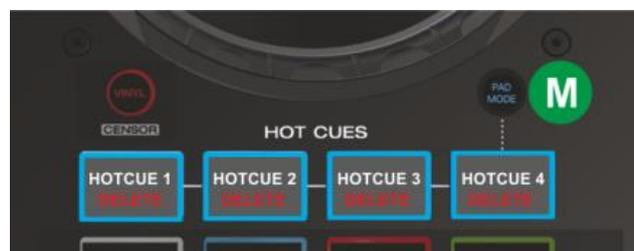
Hold **SHIFT** and then press any of the 4 Pads to **delete** its assigned Hot Cue Point.
