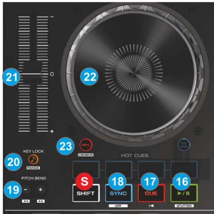
If the Deck is paused, you can press and hold the Cue Button to play the track from the Temporary Cue Point. Releasing the Cue Button will return the track to the temporary Cue Point and pause it.
