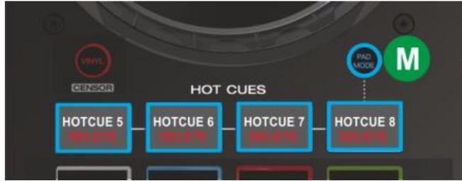
When a Pad is unlit, you can assign a Hot Cue Point by pressing it at the desired point in your track. Once it is assigned, the Pad will light up blue.
